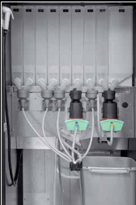
Voce Canister Layout - Triple Freshbrew Model
